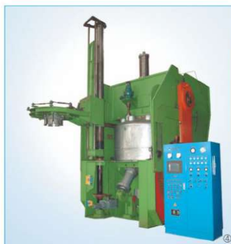
② 3500H-51VCI 液压式轮胎硫化机 3500H-51VCI Hydraulic curing press
